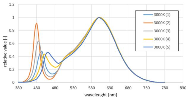
Fig. 3. Different SPDs of warm white LEDs (3000K).
