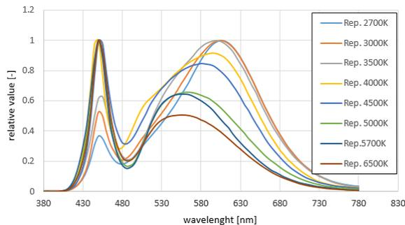
Fig. 2. The SPDs of standard white representative LEDs.
