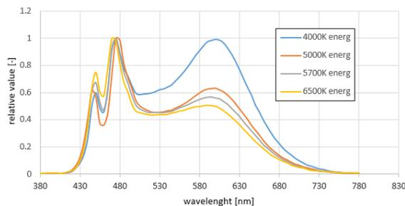
Fig. 5. The SPDs of LEDs with additional blue light radiation in the range of maximum melatopsine sensitivity (energizing).
