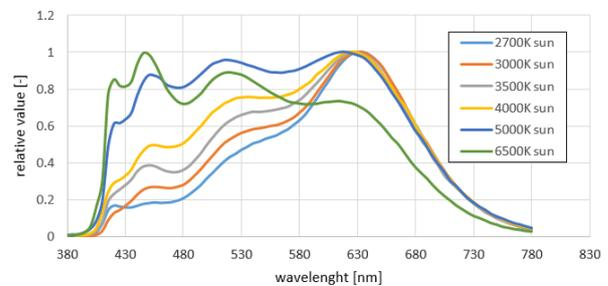
Fig. 4. The SPDs of LEDs which mimic sun light radiation in visible range.
