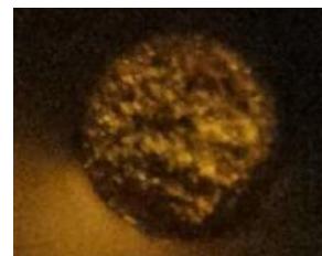
Fig. 1. Photo of the silver layer deposited on end face SMF28 optical fiber with the use of Tollens test.
