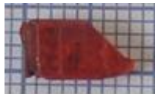
Fig. 1. (a) Scheme of synthesis of 3-ACPM; (b) Snapshot of as grown 3-ACPM single crystal.
