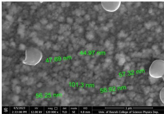
Fig. 2. SEM images of CdSe film deposited on Si wafer.
