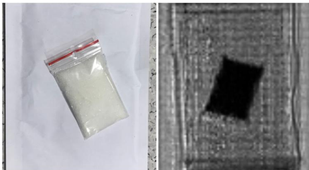
Fig. 5. Sugar sachet in an envelope (left side) and image from the scanner (right side).
