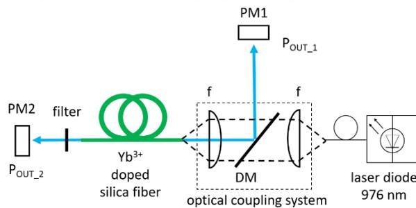
Fig. 2. The laboratory laser setup used for active fiber testing: DM – dichroic mirror,  $f$  – aspheric lenses with equal focus length, PM1 and PM2 – power meters, filter – long pass filter.
