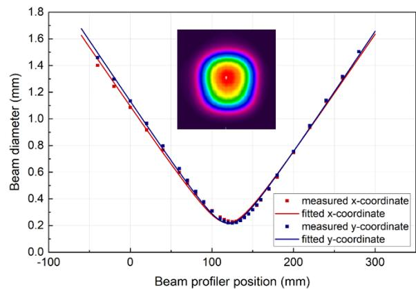
Fig. 6. The beam quality characterization;  $M_x^2 = 1.43$  and  $M_y^2 = 1.44$  were obtained at  $P_{out2}$  power of 2.38 W, registered beam profile in the waist (inset).
