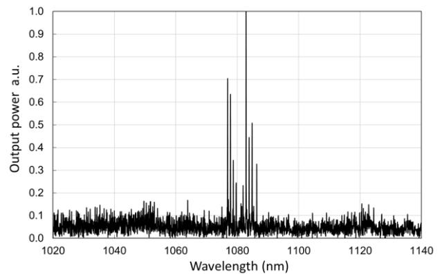
Fig. 5. The spectrum of the laser generation for 25.6 m long fiber at about 1080 nm with the FWHM = 9 nm. The spectrum was registered at  $P_{out2}$  power of 2.38 W.
