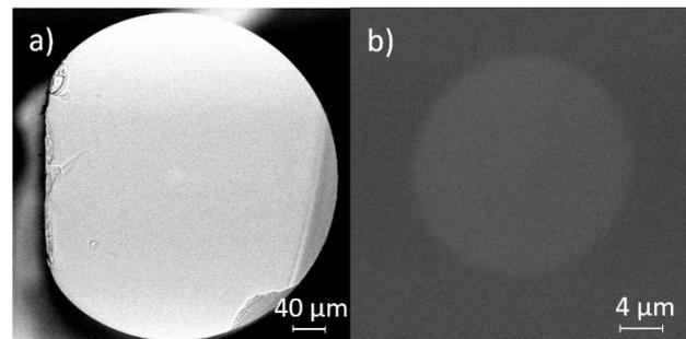
Fig. 1. SEM images of a cross-section of the fabricated Yb<sup>3+</sup>-doped fiber with a D-shape cladding with a maximum diameter of 408 μm and 362 μm on the cut side (a), and 21 μm fiber core of (bright area) (b). The shown fiber was stripped of its polymer coating.
