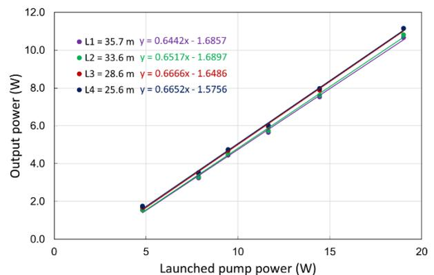
Fig. 3. The laser output power, as a sum of powers from both fiber ends ( $P_{out1} + P_{out2}$ ), versus launched pump power for several fiber lengths L1, L2, L3, and L4 tested in the laser setup. The highest efficiency of 66.7% was obtained for a fiber with a length of L3 = 28.6 m.
