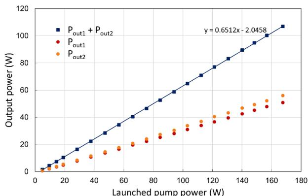
Fig. 4. The laser output power versus launched pump power for 25.6 m long fiber for up to the maximum pump power available in the laser setup. The maximum output power was 107 W, as the sum of the output powers obtained from both fiber ends  $P_{out1}$  and  $P_{out2}$ .
