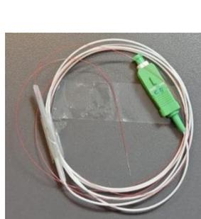
Fig. 2. Photograph of the fabricated Fabry–Pérot fiber-optic sensor.
