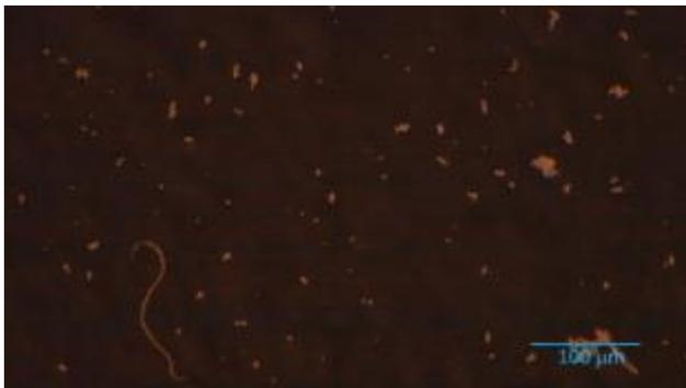
Fig. 1. Particles obtained from milling the top coat layer.
