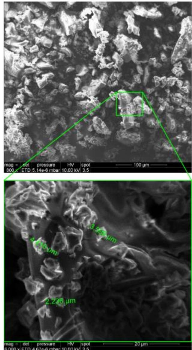
Fig. 3. SEM images of hybrid top coat particles.
