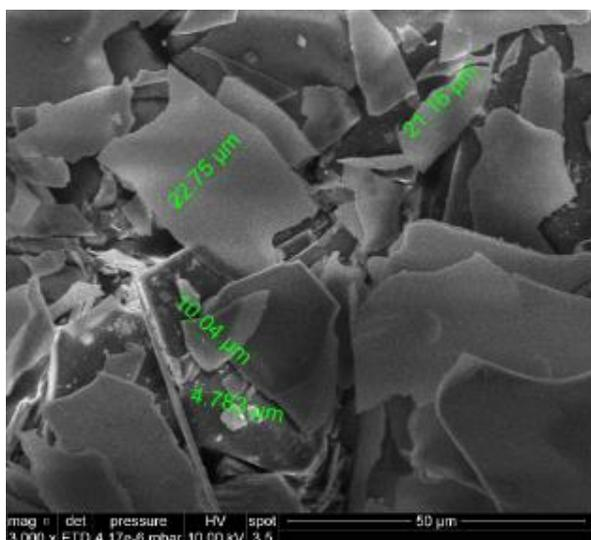
Fig. 5. SEM images of hybrid powder with irregular shape.
