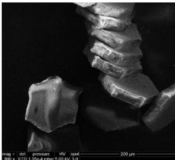
Fig. 4. SEM images of the hybrid powder with a hexagonal prism shape.
