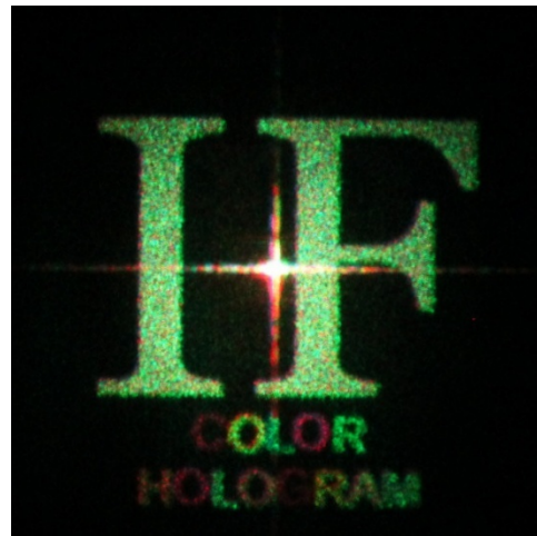
Fig. 6. Experimental reconstruction of a colour Fourier hologram with a 1/1000s exposure matched with SLM fluctuations characteristics. Suppressed 0^{\text{th}} order and inverted image from ( -1^{\text{st}} ) order.
