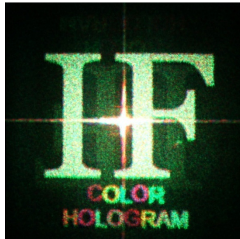
Fig. 5. Experimental reconstruction of a colour Fourier hologram with a 1/30s exposure. Disturbing 0^{\text{th}} order and inverted image from ( -1^{\text{st}} ) order.
