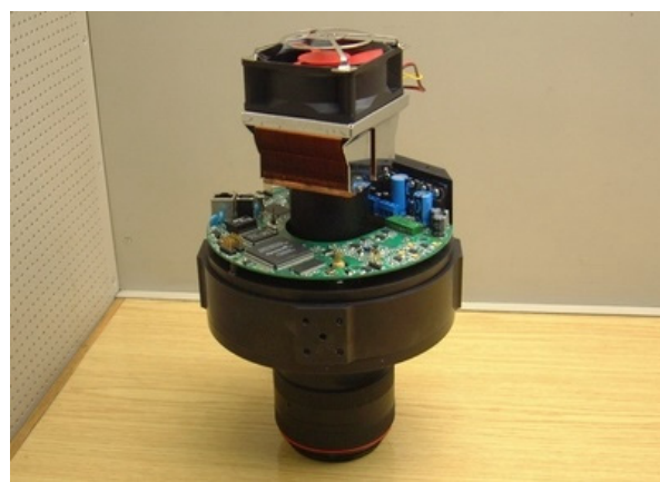
Fig. 1. Assembled K20/30 CCD camera without a cover
