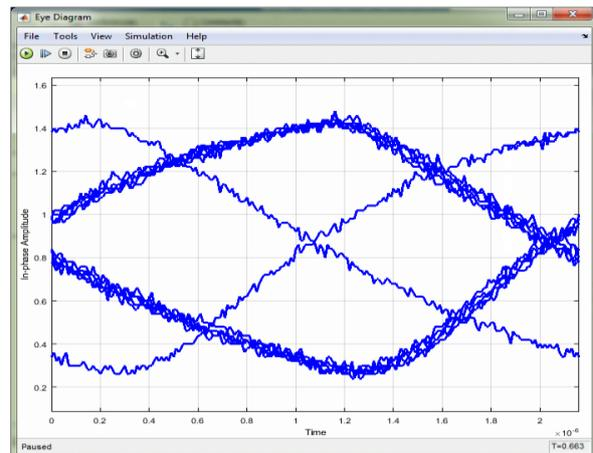
Fig. 6. Eye pattern for a bit rate of 960 kbit/s
