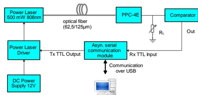
Fig. 6. Experimental set-up for BER measurement.
