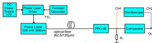
Fig.1. Optical set-up for the study of the frequency characteristics of the PPC-4E photovoltaic converter.
