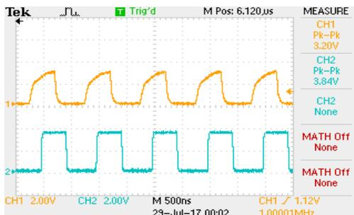
Fig. 3. Output signals from the PPC-and the from the comparator at 1MHz
