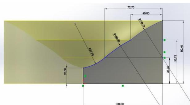
Fig. 4. Model of the mirror with a modified shape.
