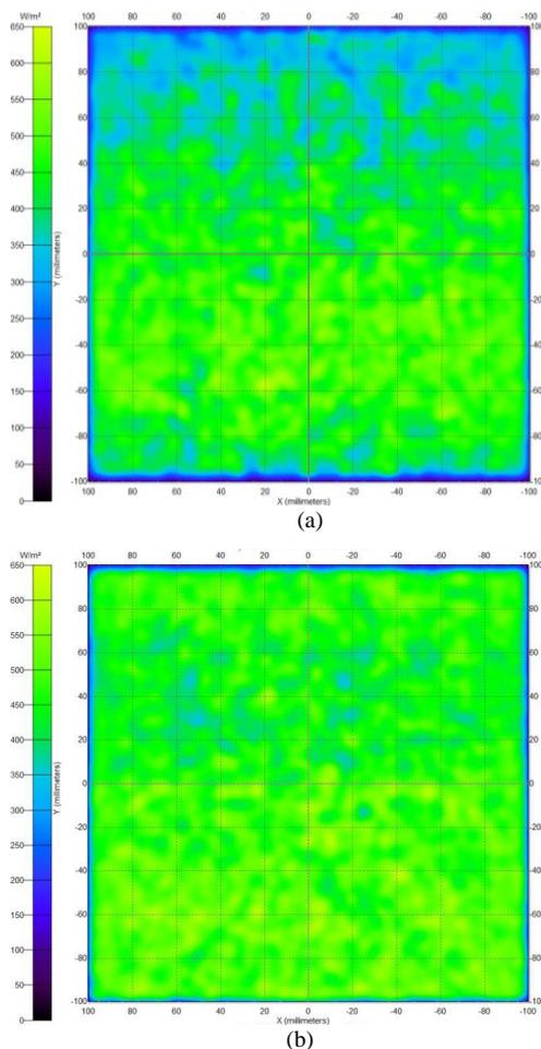
Fig. 4. Distribution of irradiance for absorbed flux in the case of the applied modified mirror surface: (a) for rays reflected by the mirror, (b)
