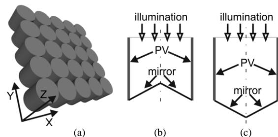
Fig. 1. Visualization of 3D solar panel module (a), the cross-section of a single-cylinder with an external (b) and internal mirror surface (c).
