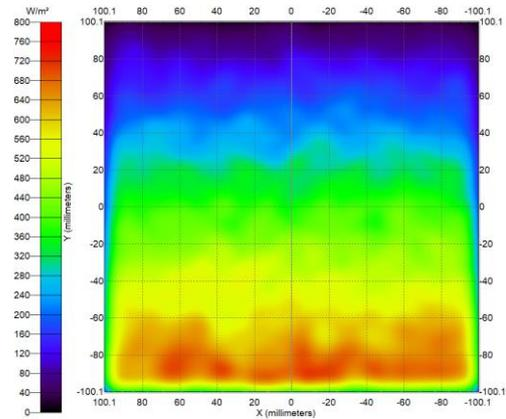
Fig. 3. The distribution of irradiance for absorbed flux at the internal surface of the cylinder after reflection from the conical mirror.
