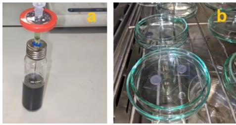
Fig. 2. (a) container with a sonicated solution before filtration through a syringe filter, (b) rGO solution after placing on a mica surface.
