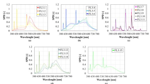
Fig. 2. The CIE fluorescent lamp illuminants: second generation classical FLs (a), deluxe FLs (b), three-band FLs (c), multi-band phosphor FLs (d), simulated the spectrum of Daylight 6504 K (e).
