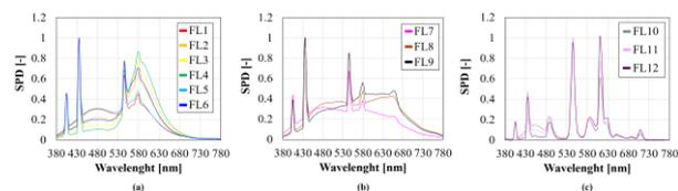
Fig. 1. The CIE fluorescent lamp illuminants: classical FLs (a), broadband FLs (b), narrowband FLs (c).
