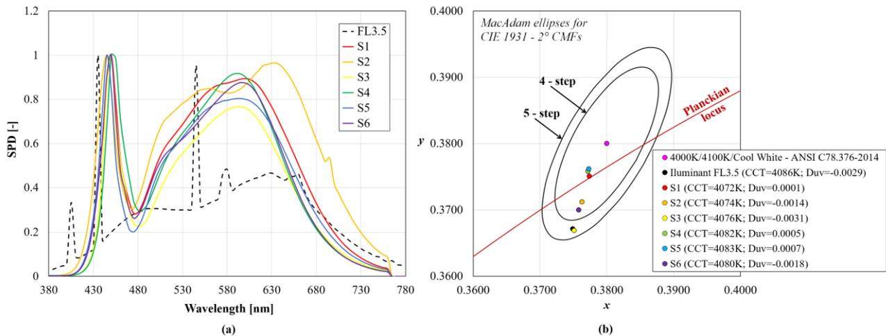
Fig. 3. Information about SPDs and  $xy$ : (a) the normalized spectral power distributions (SPDs) of the FL3.5 illuminant, LED sources and (b) the corresponding chromaticity points at CIE1931 ( $x,y$ ) chromaticity diagram.
