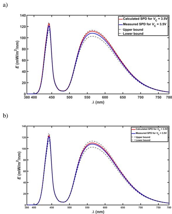
Fig. 2. Comparison of the SPD of the tested luminaire measured and calculated for  $V_C = 3.5$  V and (a) by the method using polynomial functions (b) by the method using spline functions.
