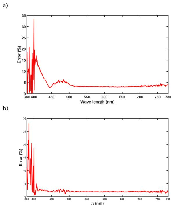
Fig. 3. Fitting error calculated for  $V_C = 3.5$  V: a) the method using polynomial functions, b) the method using spline functions.
