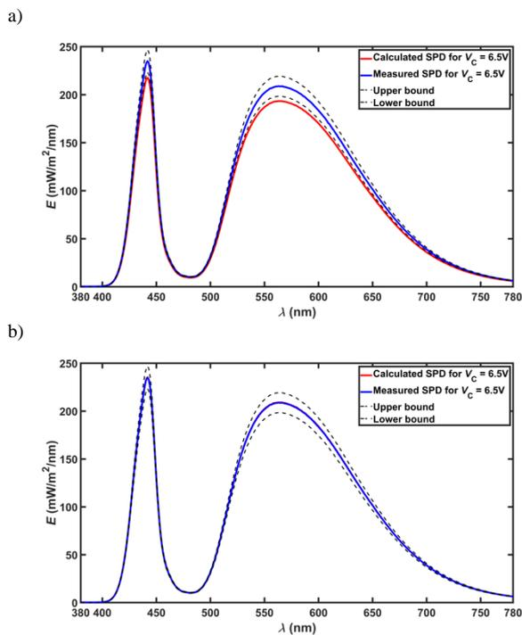
Fig. 4. Comparison of the SPD of the tested luminaire measured and calculated for  $V_C = 6.5\text{V}$  and (a) by the method using polynomial functions (b) by the method using spline functions.
