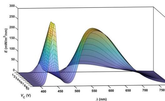
Fig. 1. The SPD of the LED luminaire in the 1–10V dimming range.
