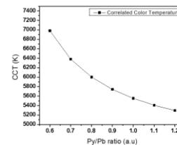
Fig. 4. CCT versus different yellow/blue power ratios.
