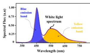
Fig. 1. White light spectrum combination from blue and yellow emission band.
