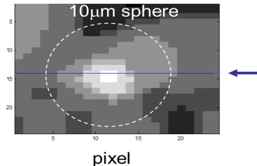
Fig. 2. Irradiance of the fringe on the microsphere.
