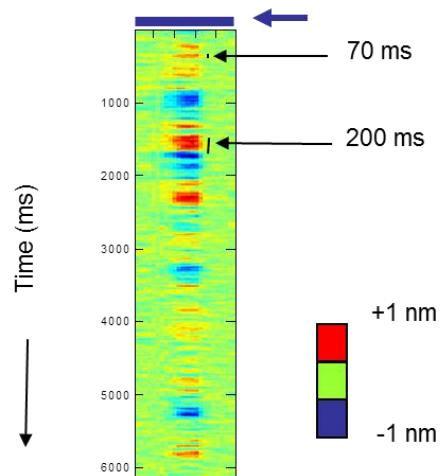
Fig. 3. The timescale of the vibrations of a sphere placed on a neuron. Vibrations are nonharmonic on nanometer order in the amplitude.
