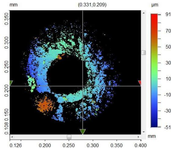
Fig. 1. Interferometric measurement of the eye of a living zebrafish embryo with a visible microsphere in a lower left corner of the eye. Patches of the reflective pigment in the iris area of the eye are visible.
