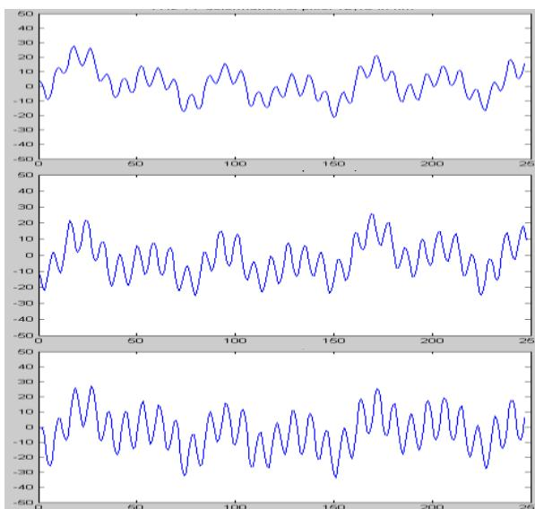
Fig. 4. 7Hz harmonic motion measured at single with 90 degree phase step algorithm and 60fps CCD camera over a period of 4 seconds. The object was moved vertically with 3 different amplitudes. The slowly varying change in amplitude is the result of the scanner nonlinearity which stays the same for each measurement. Vertical scale is in nm and lateral in pixels.
